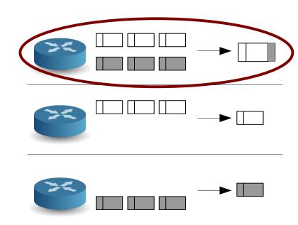
Output interface maintains real and shadow queues Q<sub>r</sub> and Q<sub>s</sub>
